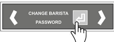
Enter the new user password using the plus and minus password and confirm it with the indicated button.
